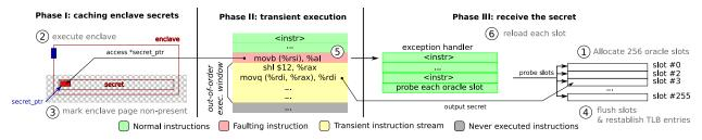
Figure 2: Basic overview of the Foreshadow attack to extract a single byte from an SGX enclave.
