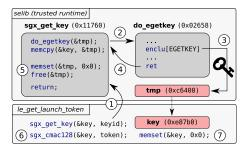
Figure 5: Key derivation in the SGX Launch Enclave.
