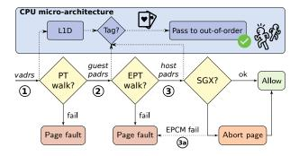
Figure 1: CPU address translation and L1 terminal fault behavior: documented architectural view (bottom) and undocumented micro-architectural transient execution interactions (top).  $^2$
