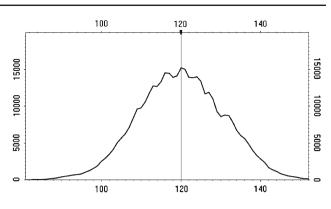
Fig. 4 Distribution of power consumption at first S-box output computation
