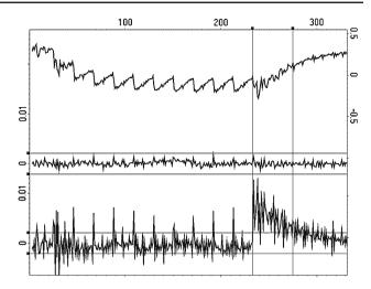
Fig. 9 DPA results showing the average trace for an AES-128 operation running on an FPGA (top), the differential trace for an incorrect guess of a byte of the last round key (middle) and the differential trace for the correct key byte (bottom)
