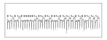
Fig. 11 SPA leaks from an RSA implementation
