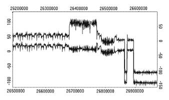
Fig. 15 A trace from a device performing RSA using CRT for which the decryption result is less than q, and a trace with decryption result greater than q
