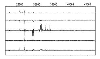
**Fig. 8** Five differential traces for the DPA test predicting the LSB of  $I_{i,0}$  for guesses  $K_0 = 101, \ldots, 105$  from top to bottom, with the correct key  $K_0 = 103$ , corresponding to the third trace
