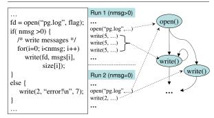
Figure 3: A sample system call graph built for the system calls shown in the middle. The program is shown on the left.
