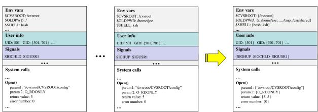
Figure 1: A simple example to show how an application signature is built from its runtime behaviors.
