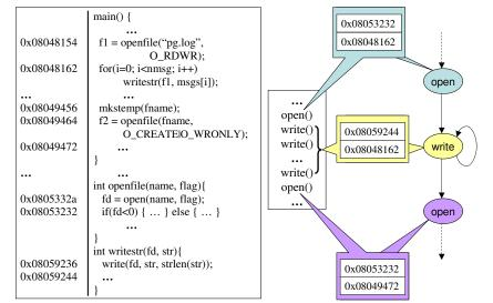
Figure 5: An example shows building system call graph with return addresses in call stack.
